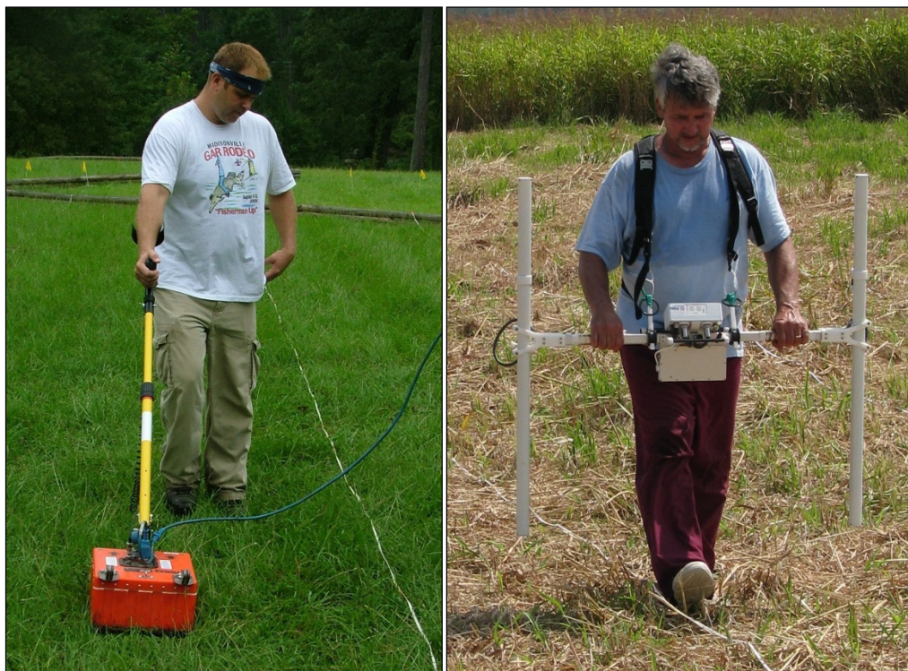
Figure 1. Use of a GSSI 400 MHz antenna detached from the SIR 3000 cart (left), and use of a Bartington Grad601 dual gradiometer (right). (Neither photo was taken during this study.)
